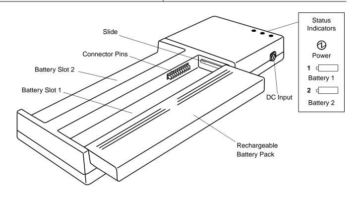
4. When the charged battery pack is needed, remove the battery pack from the charger.
